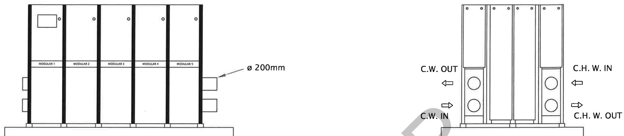
MODULAR CHILLER BANK 1
