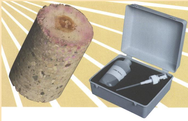
Phenolphthalein Test for Carbonation
