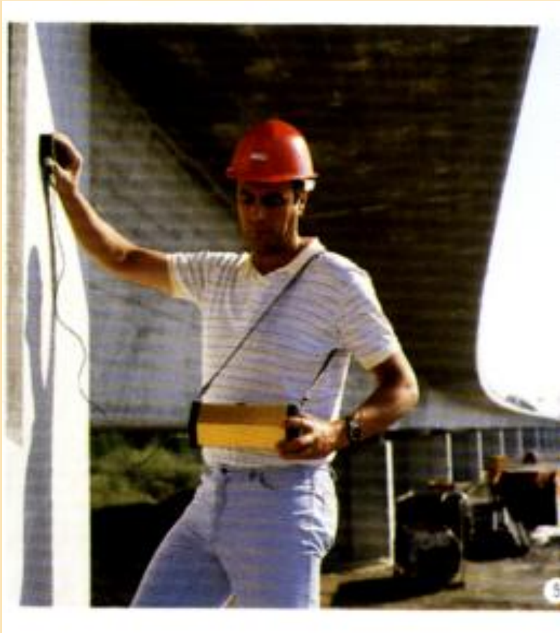
Locating the steel bars in a bridge column
