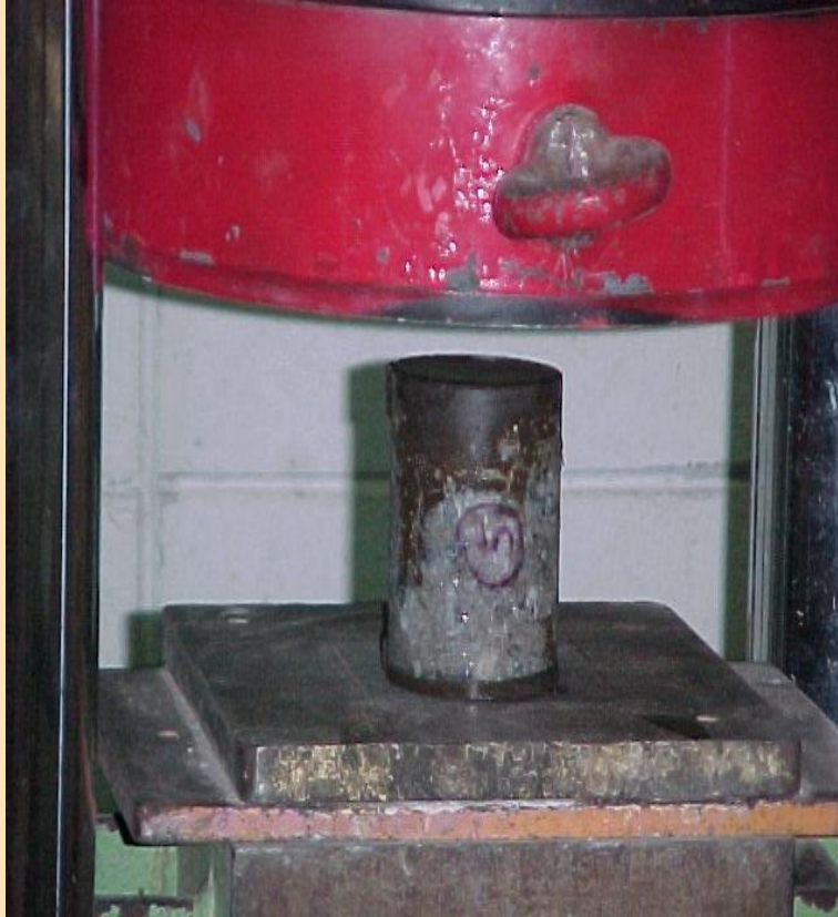
Concrete core under a compression machine
